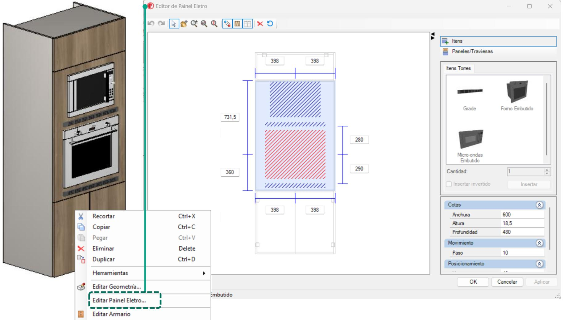
The image illustrates the process of modulating kitchen cabinets, specifically focusing on the integration of built-in appliances like ovens and microwaves. It shows a 3D perspective view of a cabinet unit and a detailed screenshot of the 'Editor de Panel Eletro' software interface.
