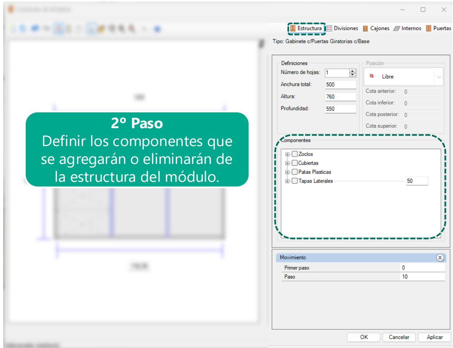
The image shows a software interface for kitchen cabinet construction. On the left, a 2D layout of a cabinet is visible with dimensions. On the right, a configuration dialog box is open, showing various settings for the cabinet structure.
