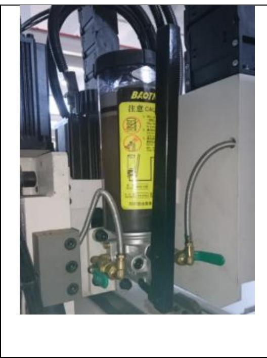
(3) Linear slide is a precision moving part which requires good lubrication in order to ensure its service life. Some sliders are connected with oil pipe supplied with oil by the electric oil pump. The other sliders unconnected with tubing should be lubricated with 0 # machinery grease by a manual grease gun once a week.
