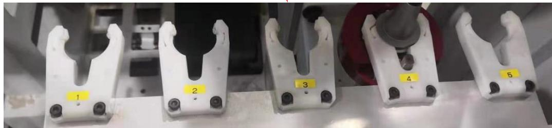
(2) If changing the tool manually is needed, switch to manual mode, move the spindle mechanism to the right side (pay attention to adjusting the spindle height and avoiding tool magazine). After confirming the spindle is not rotating, hold the knife holder by hand, and then press the button next to the tool magazine to relieve the knife.
