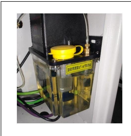
(2) Add 0# mechanical grease to manual oil pump, shake the rocker 3 to 5 times every day before working.
