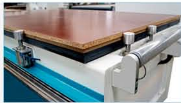
Pop-up pins for accurate positioning of workpiece
