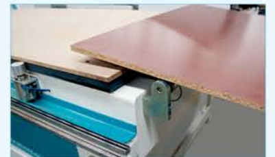
Rollers located at the front and rear end of the machine for easier loading and off-loading.
