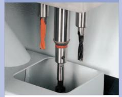
Individually selectable drilling spindles with 32 mm pitch for diverse drill diameters up to Ø 35 mm
