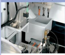
For automatic adjustment of diverse workpiece thicknesses, drilling depths and distances to the workpiece edge
