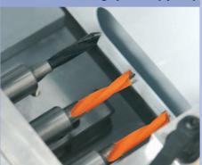
Individually selectable drilling spindles in 32 mm pitch for diverse drill diameters and doweling distances (64 mm / 96 mm)
