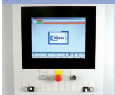
■ 15" TFT monitor ■ CD-writer ■ Modem ■ USB frontside bus ■ UPS - protects the computer against damages in case of mains interruption
